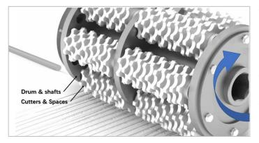
The cutting tools fix with shafts that rotates around the drum with a high speed to cut or scratch the concrete surface. The flail of cutting tool leaves a rough surface profile for various floor purposes.
